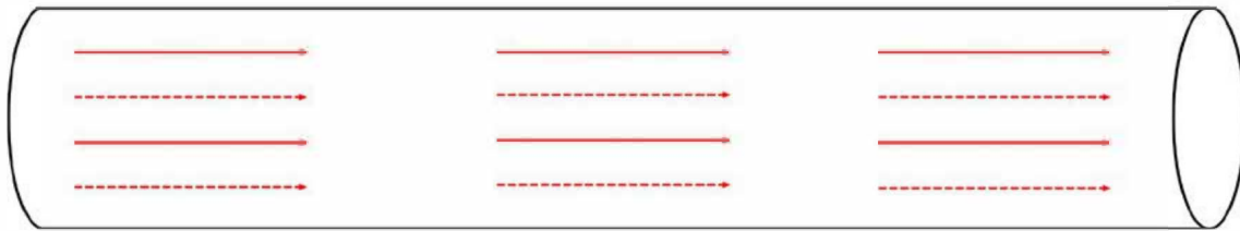
Figure A10.10.1: Four evenly spaced scanning batch measurements on a pipe diameter up to ~30 cm (~12 in) and greater than ~3 m (~10 ft) in length. Each arrow in the above diagram represents one circumferential scanning batch. Dotted arrows represent opposite side of pipe.
