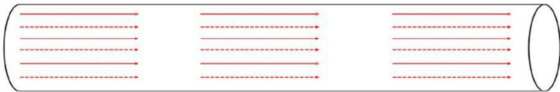
Figure A10.10.2: Six evenly spaced scanning batch measurements on a pipe diameter ~36-60 cm (~14 to 24 in) and greater than ~3 m (~10 ft) in length. Each arrow in the above diagram represents one circumferential scanning batch. Dotted arrows represent opposite side of pipe.
