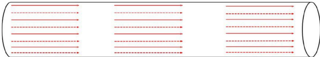
Figure A10.10.3: Eight evenly spaced scanning batch measurements on a pipe diameter greater than ~60 cm (~24 in) and greater than ~3 m (~10 ft) in length. Each arrow in the above diagram represents one circumferential scanning batch. Dotted arrows represent opposite side of pipe.
